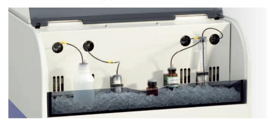
**Temperature Control & Gas Connection.** For cell based assays everything has been taken care of in order to control the internal environment. A specific incubation area ensures an extremely quick attainment and homogeneous distribution of the target temperature in the samples.
