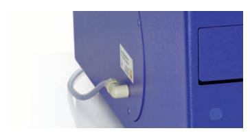
**Built-in waste pump.** For washing and filling the reagent lines you don't need to worry about loading microplates, waste containers or removal of injector tips and the built-in waste pump takes care of the safe removal of excess liquids.
