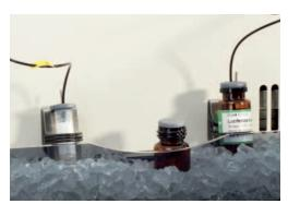
Reagent trough and holder. Space for reagent vials is available at the front of the instrument providing easy access and visibility. A removable trough can be filled with ice to keep the reagents at lower temperatures. A special reagent holder keeps small tubes, filled with valuable reagents, safely in place and ensures tubings recover the last droplet.
